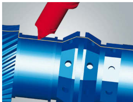
Finishing: The simultaneous movement of the B-axis allows complex contours to be finished in a single operation, preventing tool changes and mismatches
